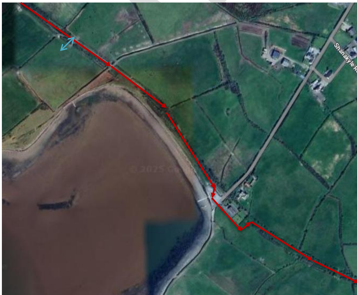
Figure 4-23 Approximate alignment in relation to Brew's Bridge with the farm overpass indicated in blue
