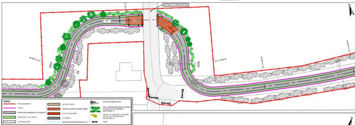
Figure 4-24 Excerpt from Drawing WCGW-ROD-HGN-S1_ML-DR-CH-200540 in Volume 3 illustrating diversion around private dwelling and crossing of local road
